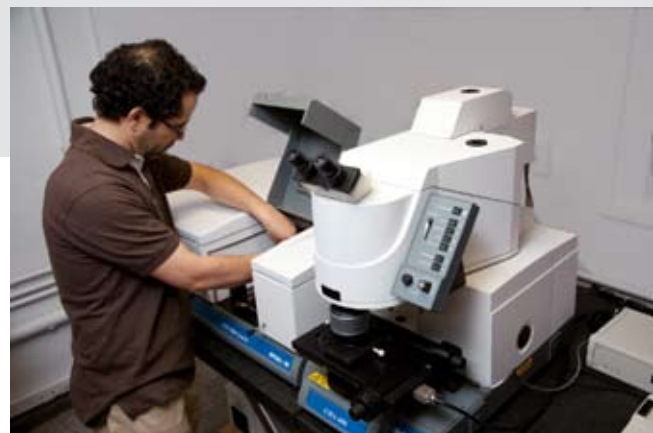
Samir Elouatik, research associate for the GCM, on a Digilab FTS7000 FTIR
