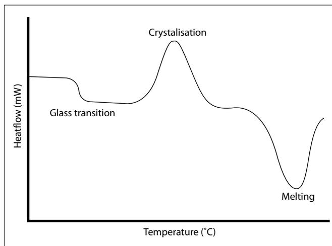
*Figure 1 : Typical characteristics of a DSC curve.*
