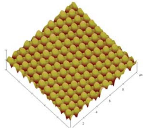
AFM image of a bilayer of polystyrene microspheres.
